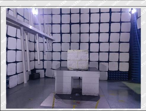
Spurious Emission Test Setup (Above 1GHz)
