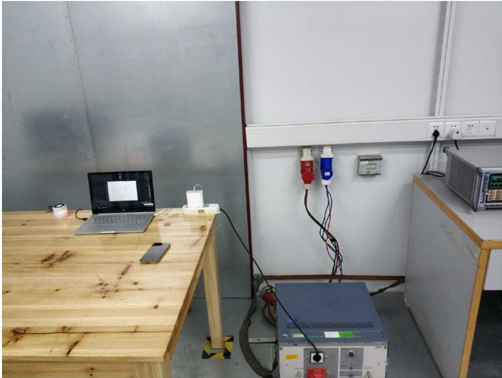
EN 55032 RADIATED EMISSION TEST SETUP
