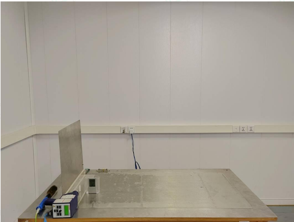
Test Setup Photo of Electrostatic Discharge Test
