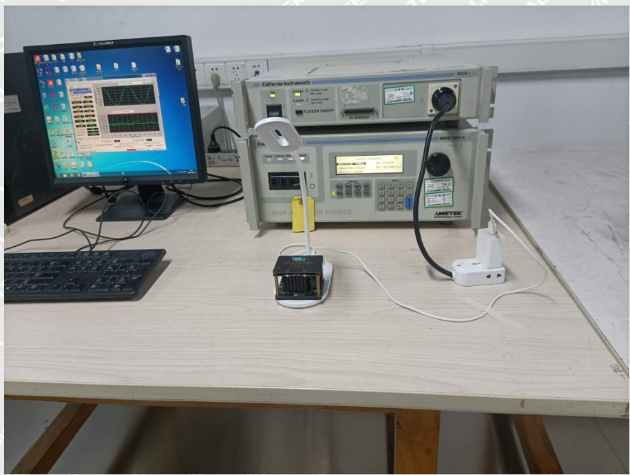
Harmonic/Flicker Test View
