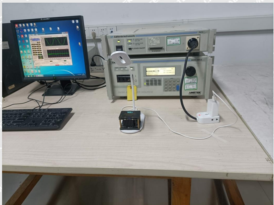
Harmonic/Flicker Test View
