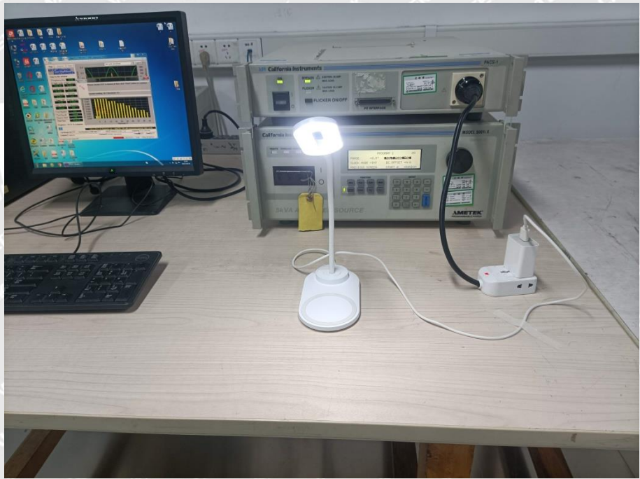
Harmonic/Flicker Test View
