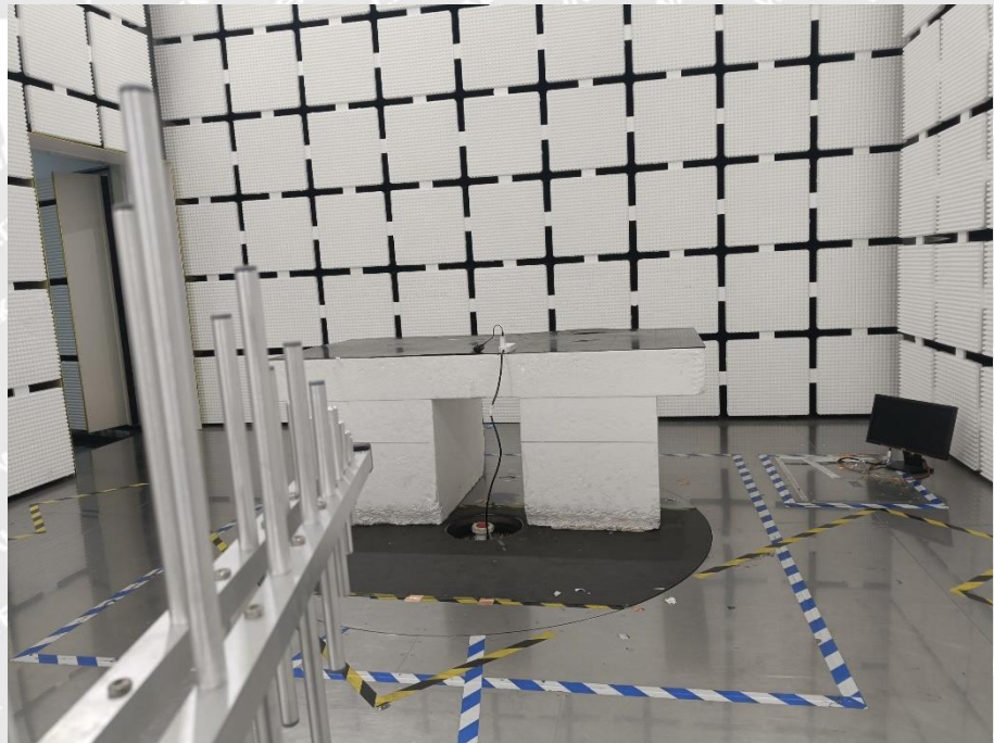
Radiation Emission Test View(30MHz to 1GHz)
