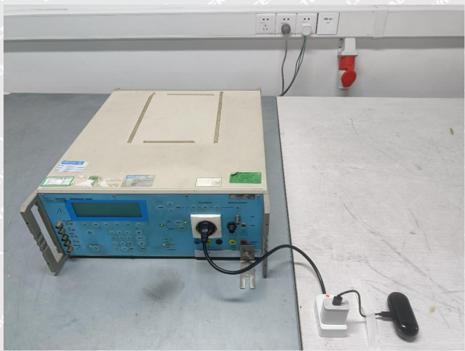
EFT/ Surges/ Dips and Interruptions Test View
