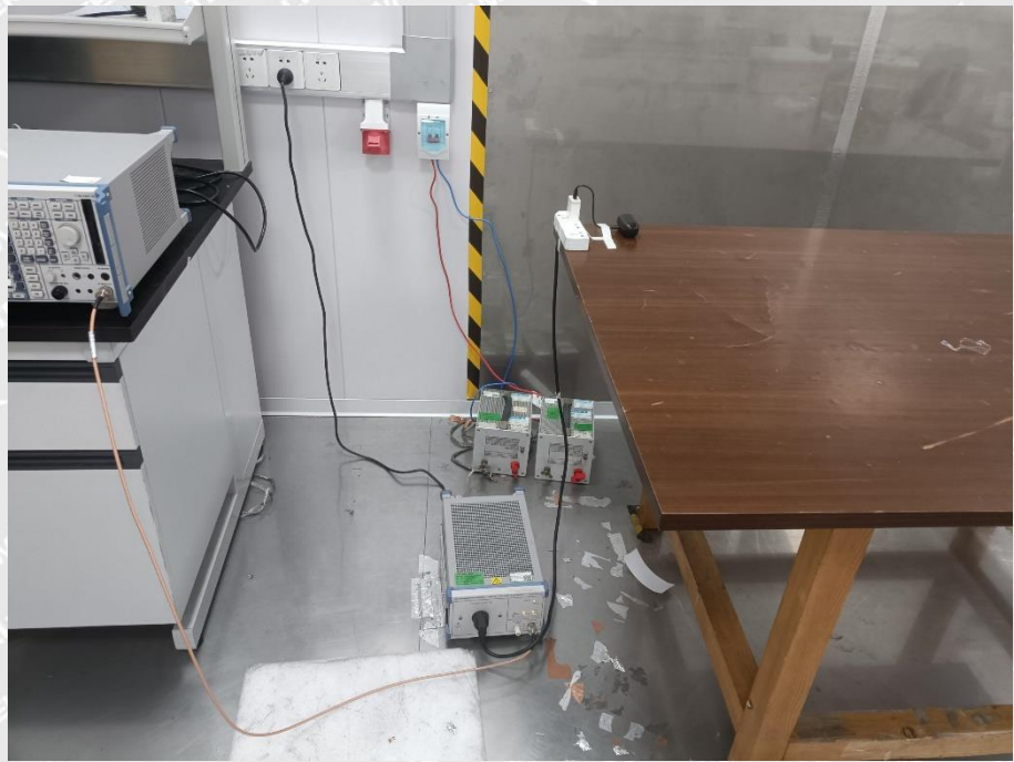
Conducted Emission Test Setup
