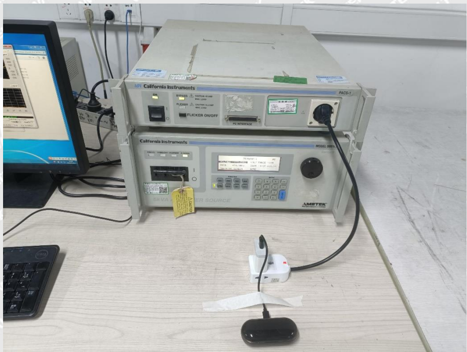
Harmonic/Flicker Test View
