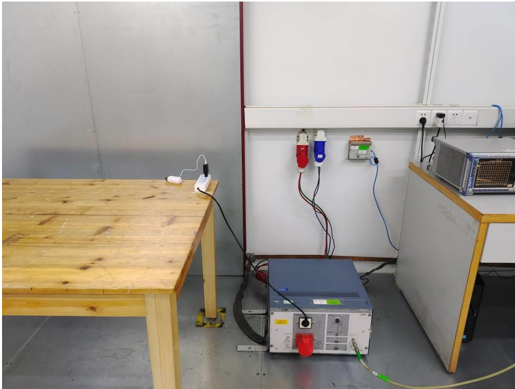
RADIATED EMISSION TEST SETUP (Below 1GHz)
