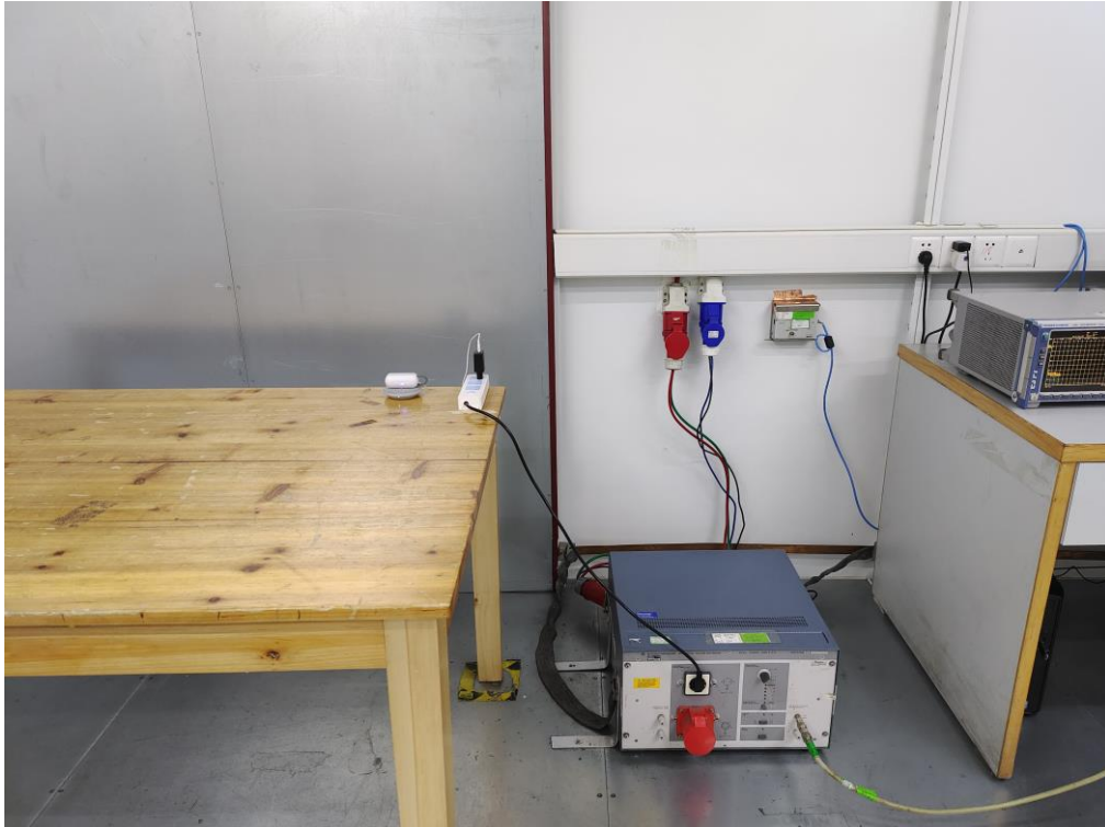
RADIATED EMISSION TEST SETUP (Below 1GHz)
