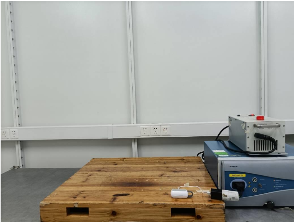
EN 61000-4-4/5/11 EFT/SURGE/DIPS IMMUNITY TEST SETUP
