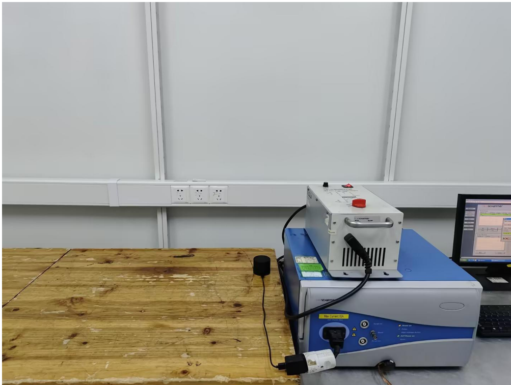
EN 61000-4-4/-5/-11 EFT/SURGE/DIPS IMMUNITY TEST SETUP
