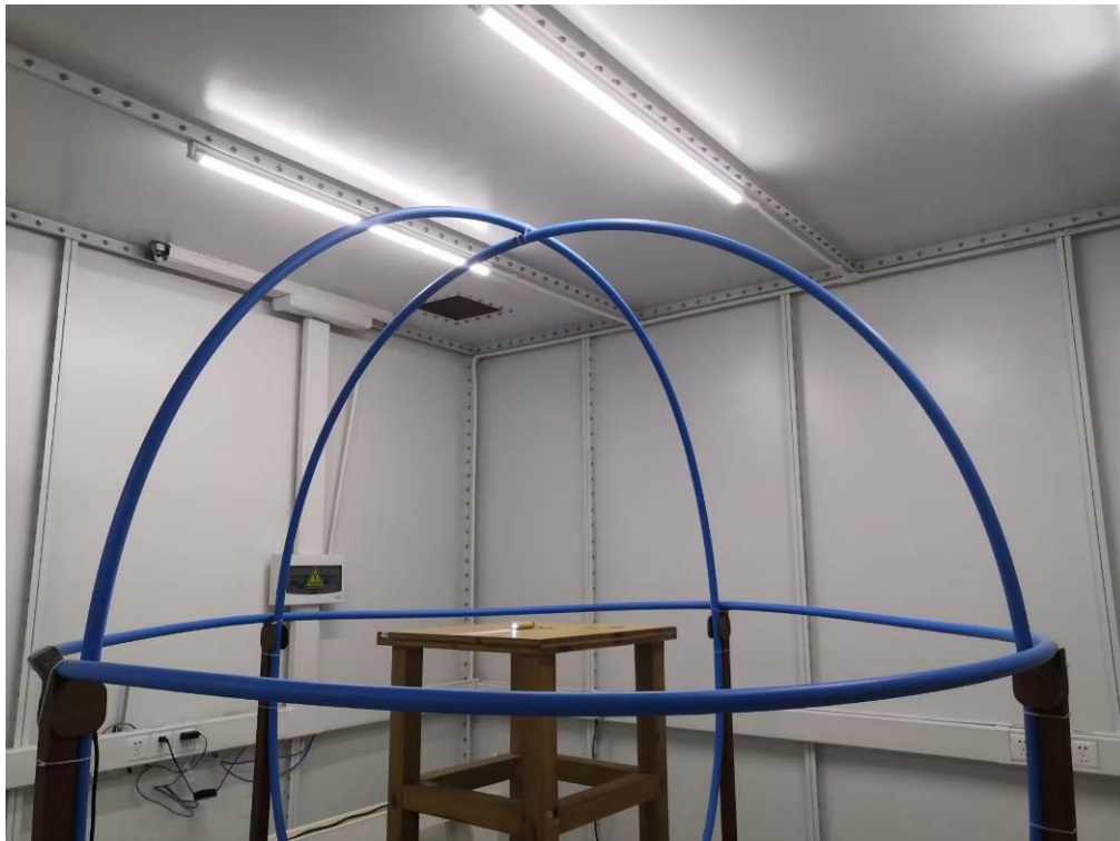
EN IEC 55015 RADIATED ELECTROMAGNETIC DISTURBANCE TEST SETUP
