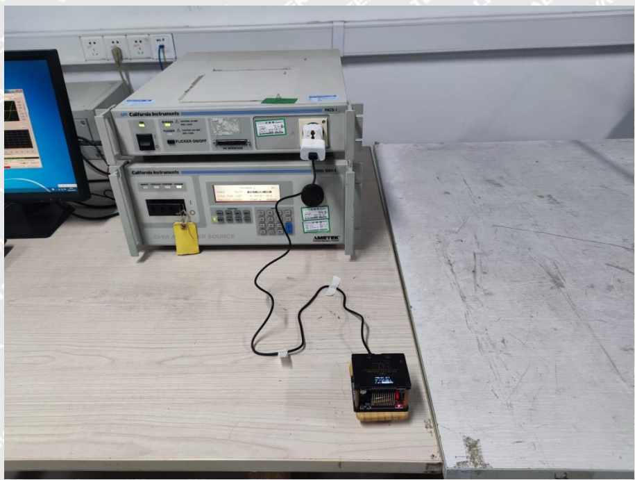
Harmonic/Flicker Test View
