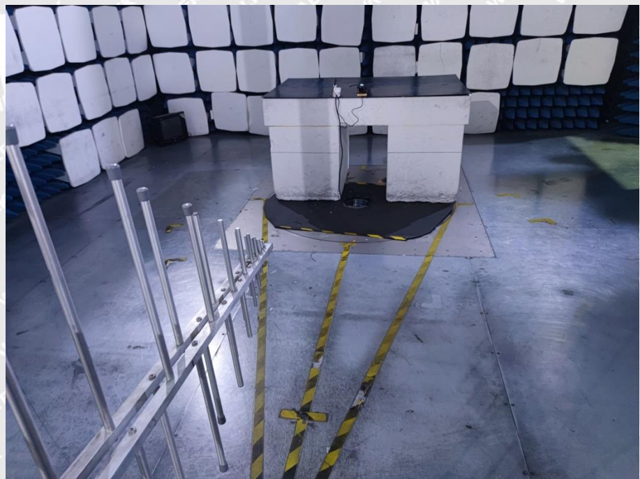
Radiation Emission Test View(30MHz to 1GHz)
