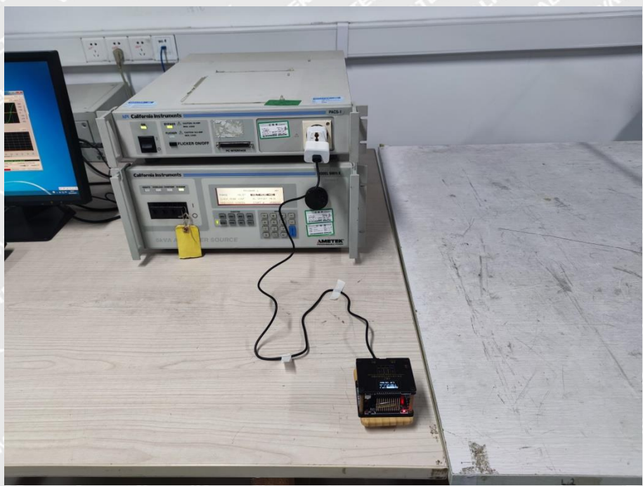
Harmonic/Flicker Test View
