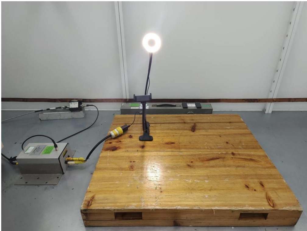
EN 61000-4-6 CS IMMUNITY TEST SETUP
