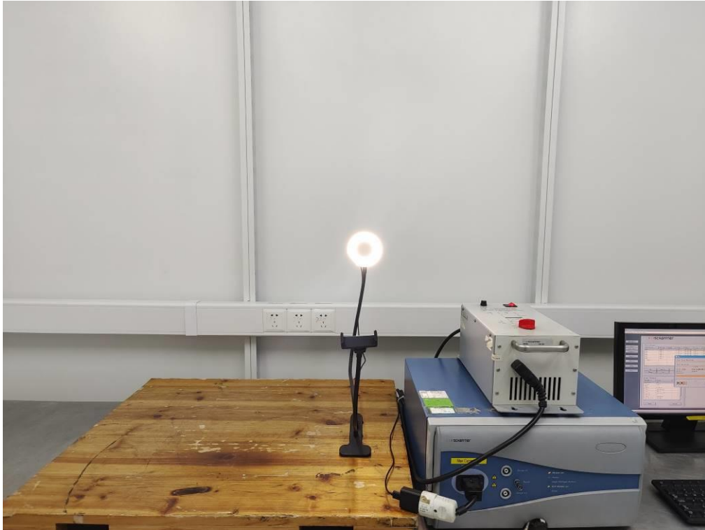
EN 61000-4-6 CS IMMUNITY TEST SETUP
