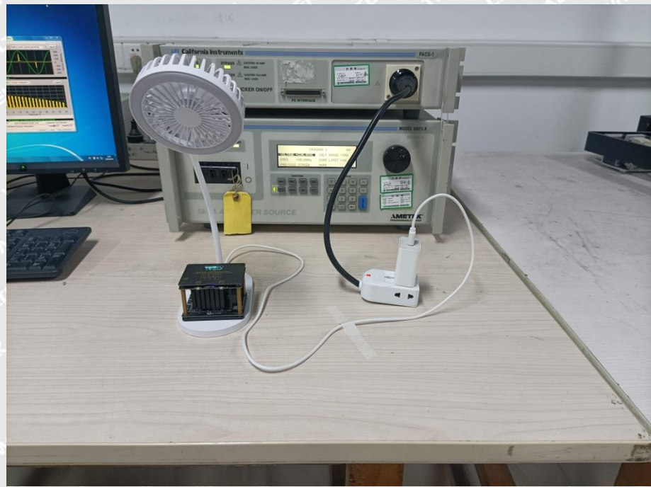
Harmonic/Flicker Test View
