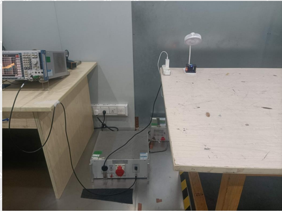
Conducted Emission Test Setup
