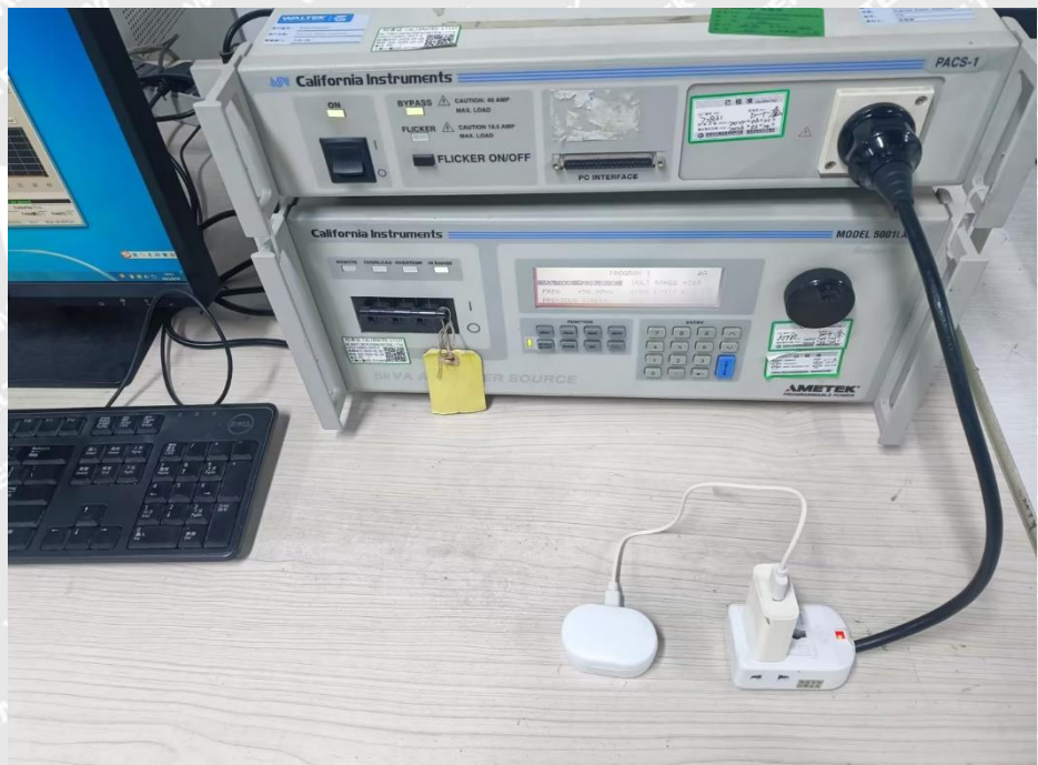
Harmonic/Flicker Test View
