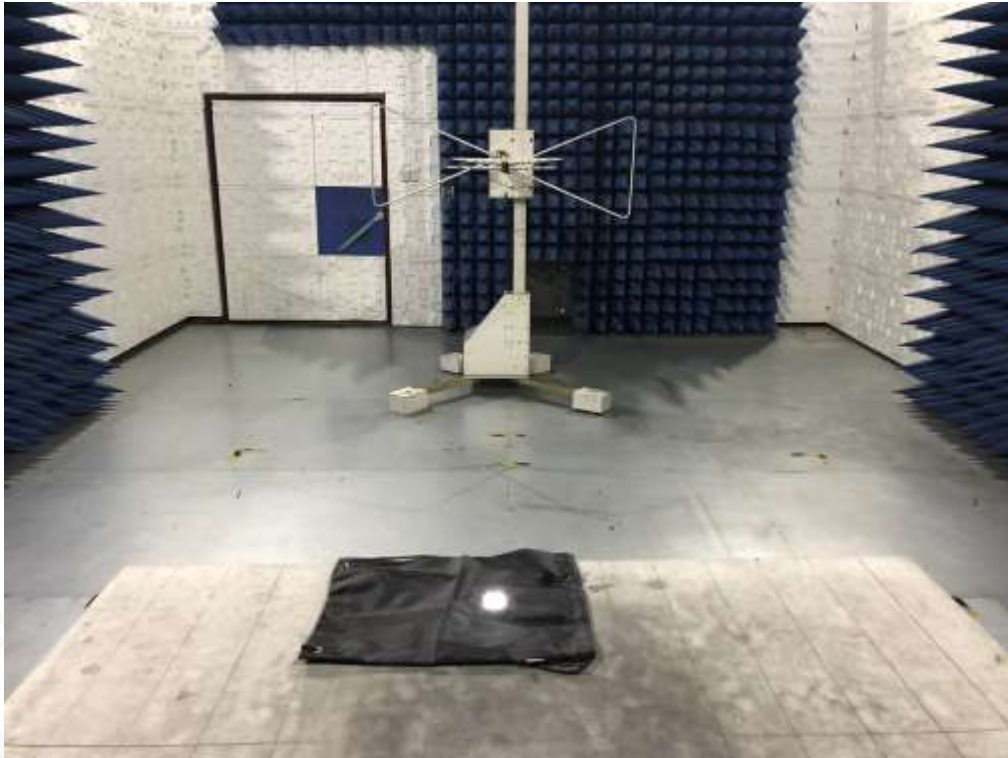
EN 55015 RADIATED ELECTROMAGNETIC DISTURBANCE TEST
