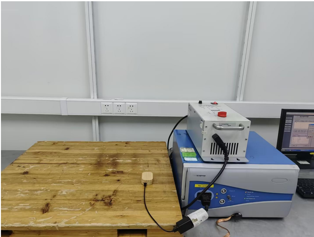
EN 61000-4-4/5/11 EFT/SURGE/DIPS IMMUNITY TEST SETUP
