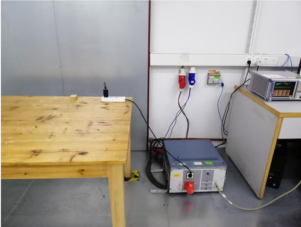
RADIATED EMISSION TEST SETUP (Below 1GHz)
